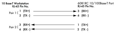
Figure 9. Cross-over RJ-45-to-RJ-45 Ethernet cable diagram
